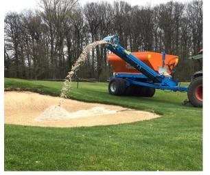
With four different hopper capacities and trailed and mounted models, there's a GKB Sandspreader to suit all surfaces. Delivering the ultimate versatility for broadcast topdressing, it is the fast and effective way to incorporate sand into greens,
